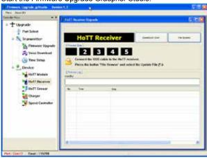
Under "Port Select" select the correct COM port "Silicon Labs CP210x USB to UART Bridge", i.e. the one to which the USB lead is connected.
